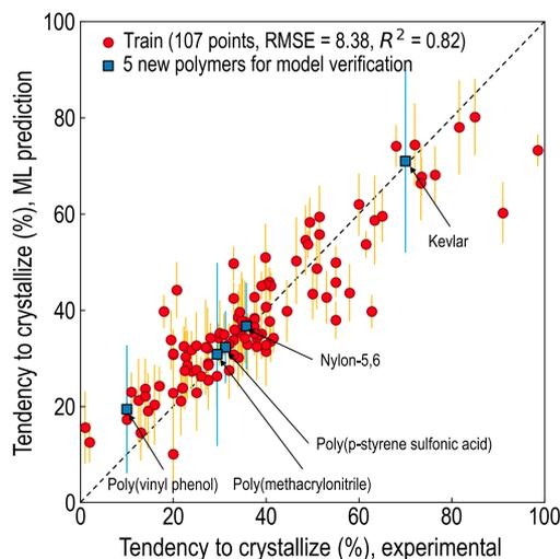
**Figure 6.** Validation of the multifidelity cokriging model using five new polymers whose experimental percent crystallinity values are compared with its predicted values.
