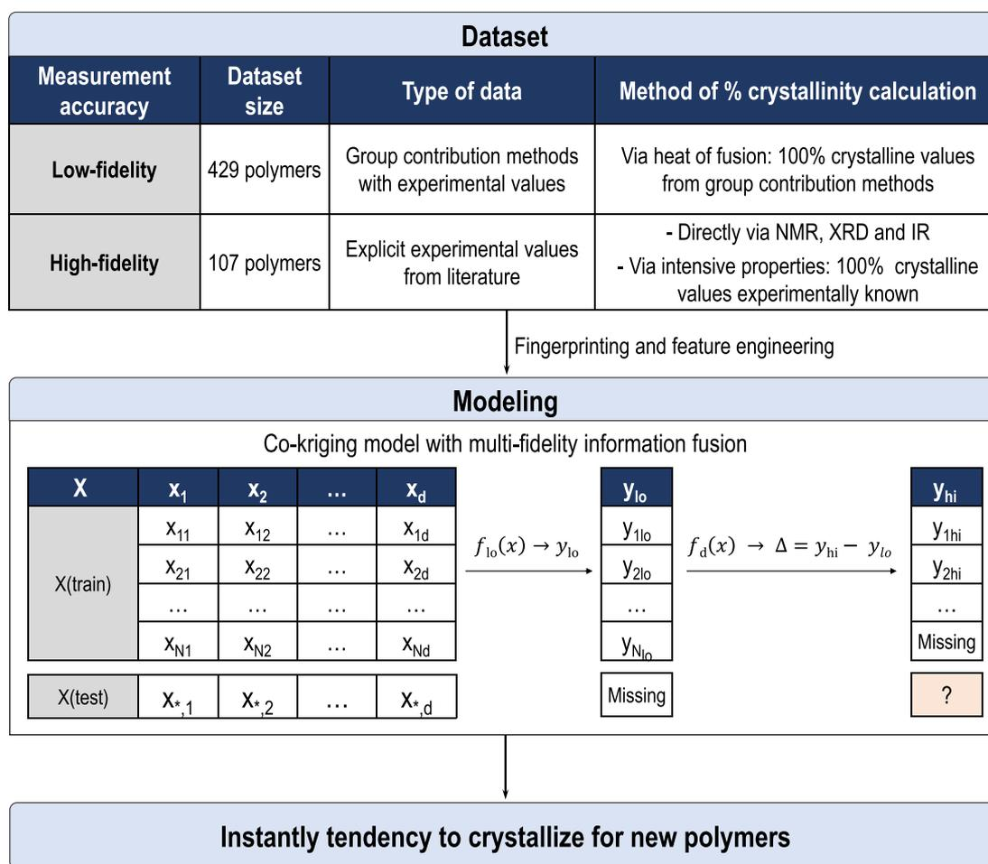
**Figure 1.** Workflow schematic used to instantly predict the crystallization tendencies for new polymers.
