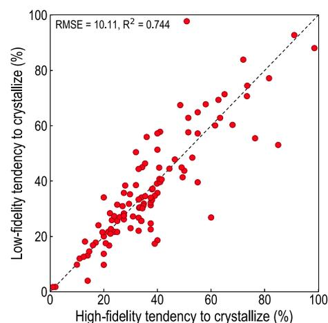
**Figure 4.** Prediction capability of the group contribution method for crystallization tendencies as a function of the high- and low-fidelity data sets.
