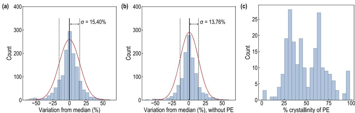
**Figure 2.** Capturing the variability of the high-fidelity data set due to polymer processing. (a) Normal distribution fit for variation from median for 30 polymers with multiple reported values of percent crystallinity. (b) Normal distribution fit for variation from median for 29 polymers, without polyethylene with multiple reported values of percent crystallinity. (c) Percent crystallinity values of polyethylene for 229 distinct samples.
