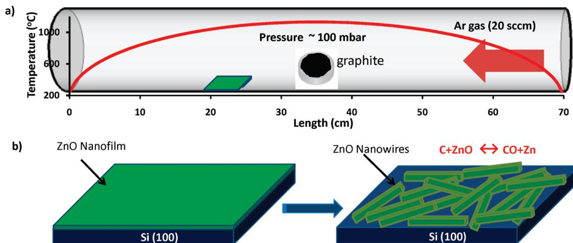
**Figure 1.** (a) Schematic diagram of the in situ carbothermal ZnO nanowires growth setup. (b) Schematic diagram of in situ ZnO nanofilm (i) conversion into ZnO nanowires and (ii) in the presence of appropriate gas flow.
