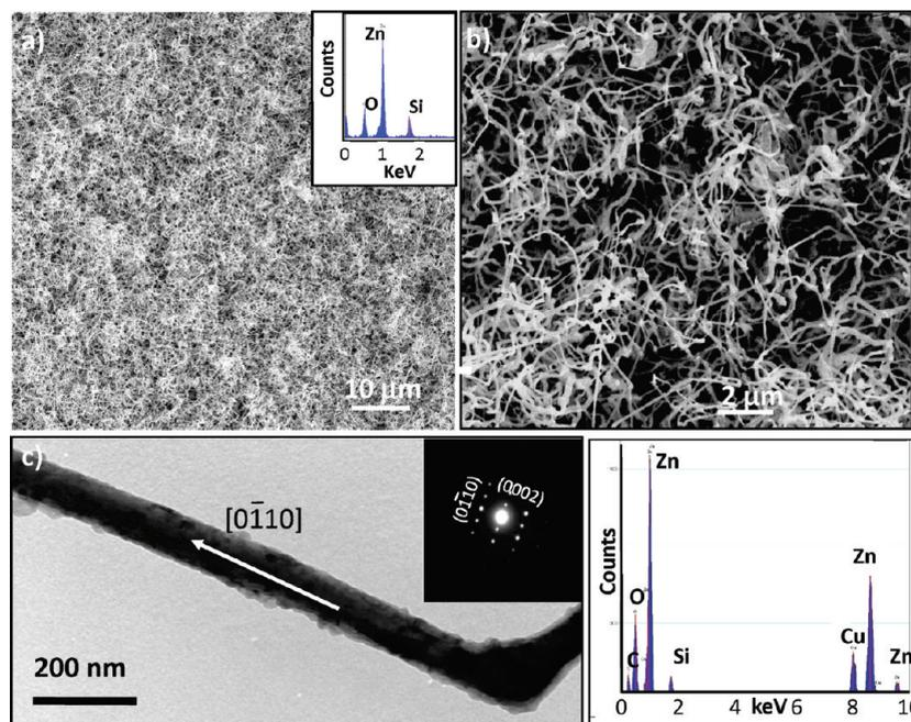
**Figure 2.** (a) Typical low magnification SEM image of zigzag ZnO nanowires. Inset in (a): the EDX spectrum of ZnO nanowires, (b) a high magnification SEM image of zigzag ZnO nanowires, (c) a representative TEM image of ZnO nanowire and the corresponding selected area electron diffraction (SAED) pattern (inset in c), and (d) a typical EDX spectrum of single nanowire in TEM.
