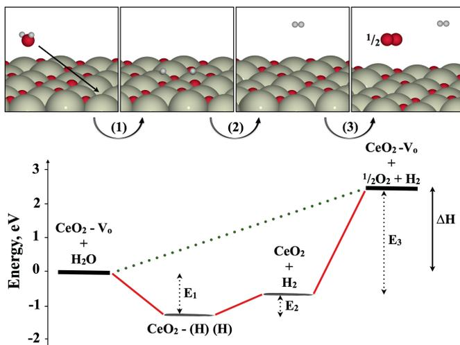
**Fig. 8.1** Reaction pathway and energetics (*red solid line*) for the dissociation of  $\text{H}_2\text{O}$  on an undoped ceria surface.  $\text{CeO}_2\text{-V}_\text{o}$  is an oxide with a vacancy,  $\text{CeO}_2\text{-(H)(H)}$  is an oxide with vacancy filled by a  $\text{H}_2\text{O}$  molecule and  $\text{CeO}_2$  is a stoichiometric surface. The *green dotted line* shows the minimum energy pathway for dissociation. Ce, O and H are represented by beige, red and white colors respectively
