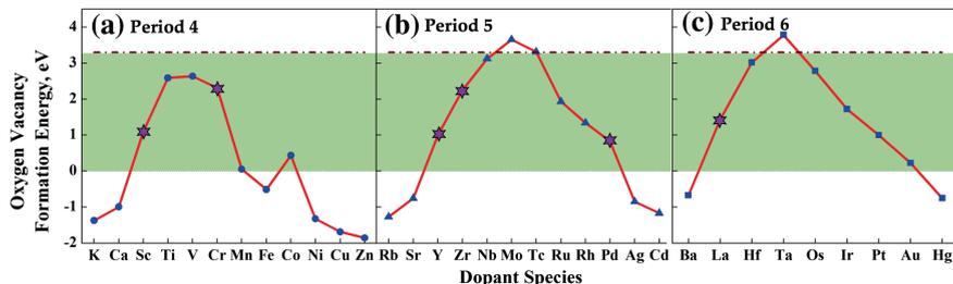
**Fig. 8.2** Oxygen vacancy formation energy ( $E_3^D$ ) of doped ceria with elements from the (a) 4th, (b) 5th and (c) 6th period of the Periodic Table. *Dot-dashed maroon line* indicates  $E_3^D$  for undoped ceria. *Light green region* indicates dopants that survived *Criterion 1*, while  $\star$  identifies dopants that survived the 3 screening criteria
