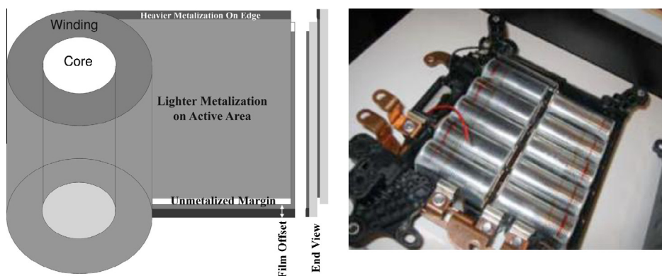
Fig. 2. (Left) Single-section winding showing more heavily metallized edges region, lightly metallized active region, and an unmetallized margin. The two layers are offset so that the heavily metallized region at the top protrudes beyond the layer below. (Right) A bank of metallized capacitor windings found in a typical hybrid electric vehicle.
